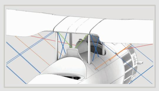
• We recommend Type B, Type C and Anchor points 1/48 Gaspatch metal turnbuckles.
