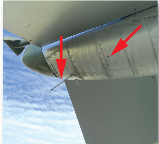
On this F-4C you can see the patch over the original location, and the TCTO version that replaced it.
