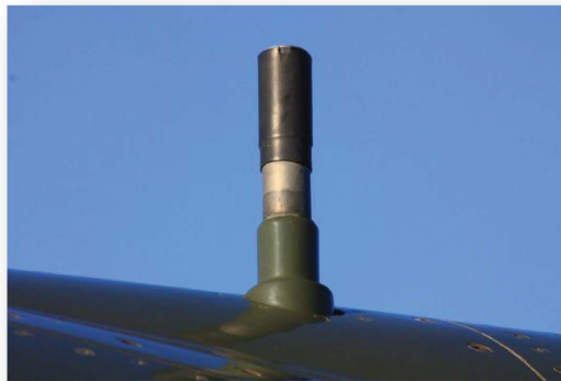
This photo shows the F-4E factory installation. Note the varying diameters of the antenna, and the black neoprene boot covering about 2/3 of its length. The green camouflaged portion is the mounting stub.
