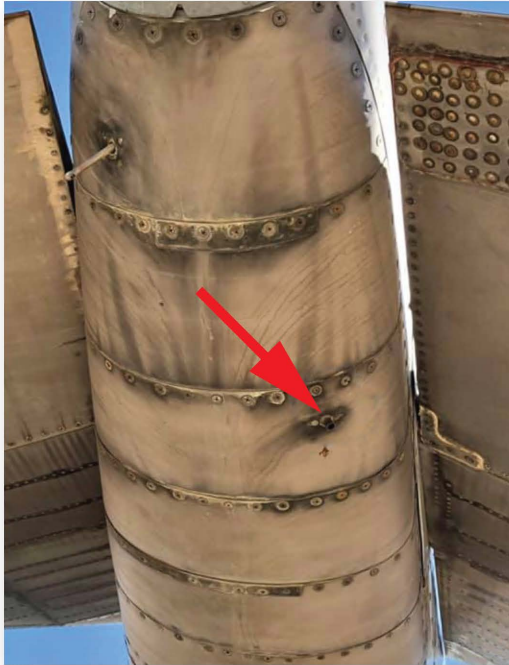
The original style and location for the vent tube is seen on this YF-4J (built as an F-4B). The handle above and to the left is the manual drag chute door release, found on all Phantoms.
