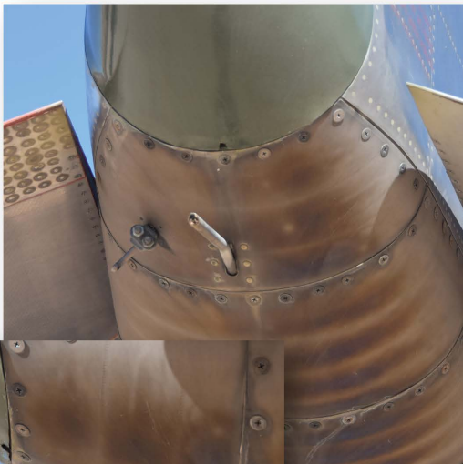
Three photos of the revised vent tube on F-4C-22-MC 64-0673. Note that it is slightly left of centerline, and how the tip is angled to be basically parallel with the bottom of the fuselage structure in this area.
