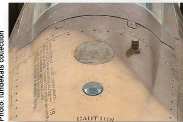
This photo shows the F-4E factory installation, with just the mounting stub, but no SST-181 antenna fitted.
