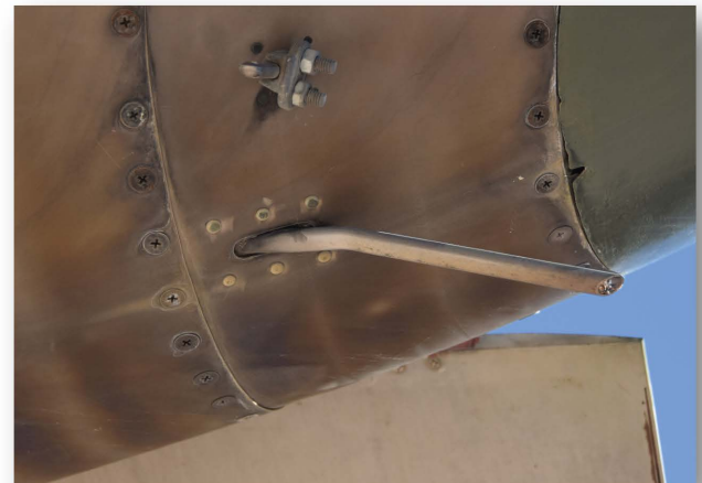
On this F-4C you can see the patch over the original location, and the TCTO version that replaced it.
