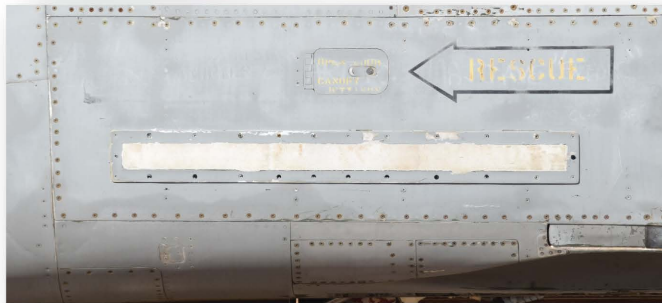
Left: the forward fuselage light on QF-4E-61-MC 74-1625 showing the slight raised frame.
