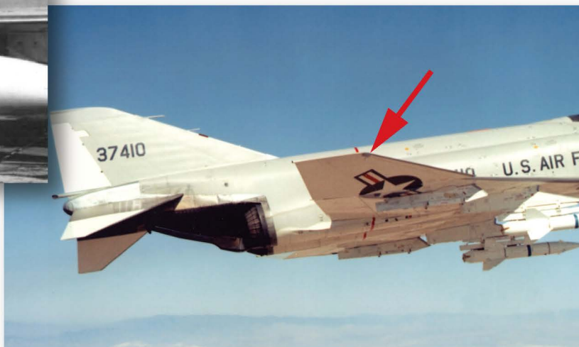
Right: F-4C-15-MC 63-7410 showing the flush style lights.
