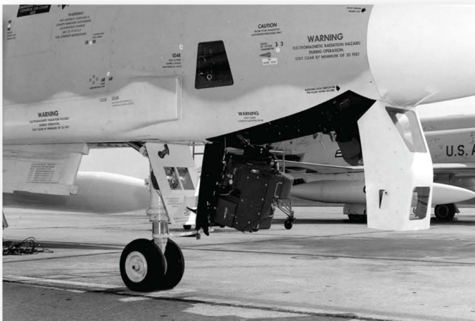
Left: an early RF-4C in the Light Gull Gray over white scheme on the ramp in St. Louis showing the white dots between or near the Access Door markings.
