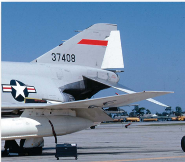
Below: F-4C-15-MC 63-7408 photographed during 1965, now with the 'bug eye' style nav lights.
