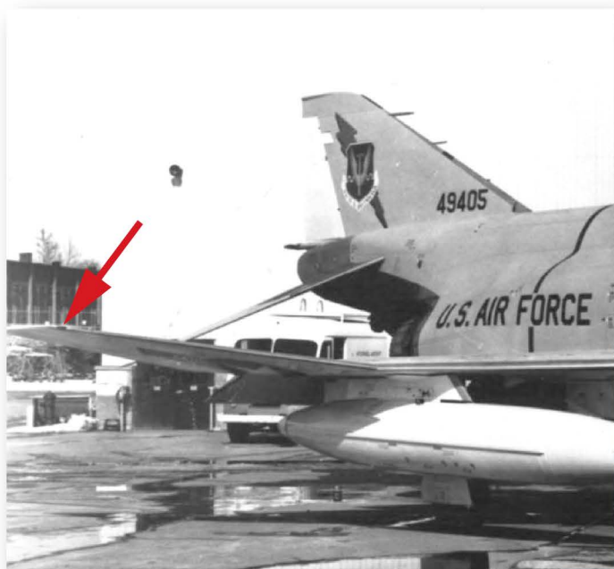
Left: F4H-1 149405 Block 9, alias F-110A is seen shortly after roll out in Jan 62. She has the original flush style nav lights.
