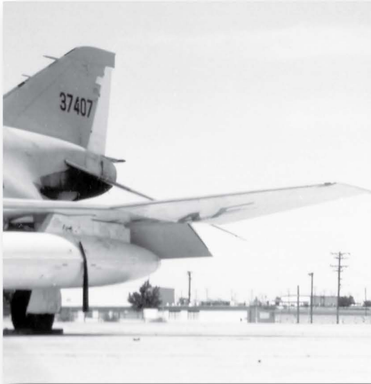
Above: F-4C-15-MC 63-7407 displays the flush style light shortly after roll out in Jul 63.
