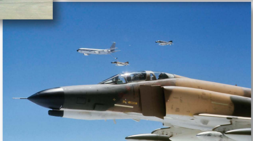
Above: Iran's initial F-4E deliveries were -46 and -47-MC blocks with FY69 USAF serials, delivered between Mar and Nov 71. As such, these were all hard wing aircraft, and survivors were upgraded with slats in 1973-74. Many continue in service with the IRIAF today after having served for over 50 years and participated in at least two wars - the Dhofar War of 1973-76 in Oman and the Iran-Iraq war of 1980-88.
