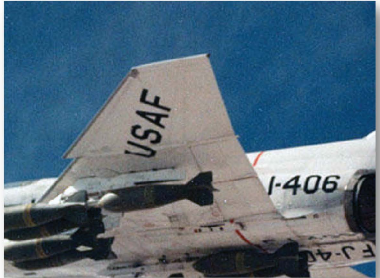
Above: We can't explain how F4H-1 149406 Block 9, here marked as the second F-110A prototype, got the later 'bug eye' lights as quickly as it did, but photos don't lie! This photo dates from the summer of 1962 during weapons compatibility testing.
