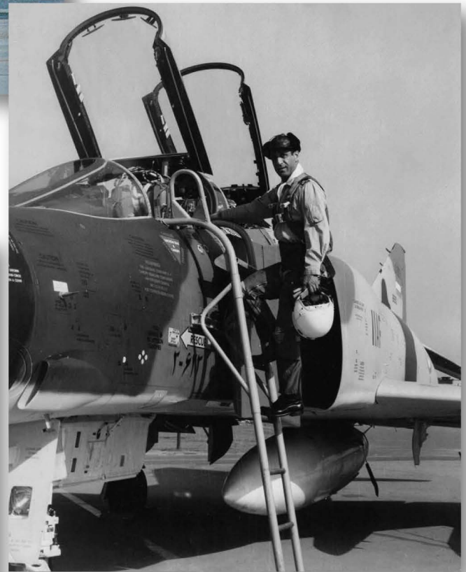
Right: IIAF Commander-in-Chief Gen. Khatami climbs aboard F-4D-37-MC 68-6910 (3-623), delivered 7 Jul 69. Absolutely standard factory 'Asia Minor' camouflage and stencils. Note the very visible internal canopy fiberglass sealing strips.
