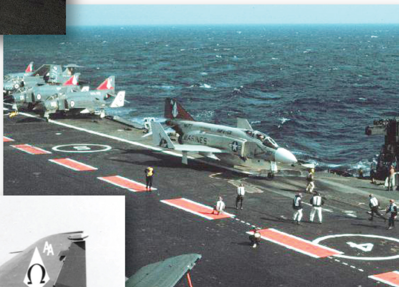
Above and right: AA 207 was eventually repaired and prepared for launch back to her home base aboard USS Forrestal. She is seen here being towed into position and then bridled to the waist catapult on the Ark Royal. The catapult on the Ark was always marginal at best for an aircraft the size of a Phantom, but the Brits made it work! Royal Navy FG.1s had a double extension oleo nose gear strut to give them a higher angle of attack on launch, something no U.S. Phantom had, so launching from the Ark must have been exciting!
