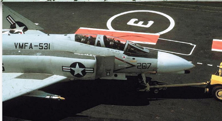
Above and right: AA 207 was eventually repaired and prepared for launch back to her home base aboard USS Forrestal. She is seen here being towed into position and then bridled to the waist catapult on the Ark Royal. The catapult on the Ark was always marginal at best for an aircraft the size of a Phantom, but the Brits made it work! Royal Navy FG.1s had a double extension oleo nose gear strut to give them a higher angle of attack on launch, something no U.S. Phantom had, so launching from the Ark must have been exciting!
