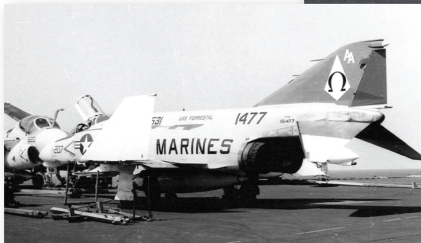
Above and right: AA 207 was eventually repaired and prepared for launch back to her home base aboard USS Forrestal. She is seen here being towed into position and then bridled to the waist catapult on the Ark Royal. The catapult on the Ark was always marginal at best for an aircraft the size of a Phantom, but the Brits made it work! Royal Navy FG.1s had a double extension oleo nose gear strut to give them a higher angle of attack on launch, something no U.S. Phantom had, so launching from the Ark must have been exciting!
