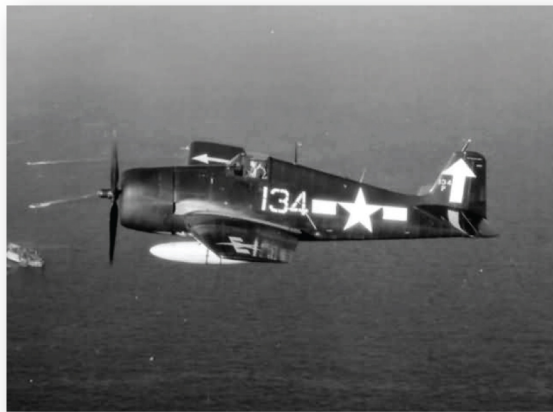
132's sister ship is airborne over the fleet. Note her lack of a left side oblique camera mount and the associated upper wing sighting markings. We believe this type of F6F-5P had a lower fuselage trimetrogon mapping camera mount as some F6F-3Ps did, but we have not been able to find absolute proof of this. Note the high gloss finish and the general lack of weathering other than the brownish-grey (tetraethyl lead) exhaust staining.
