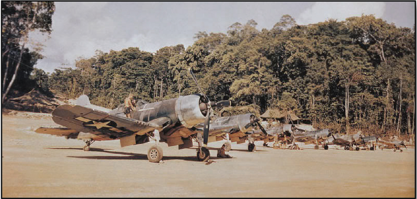
This photo shows the abysmal condition of Corsairs involved in hectic combat operations in the Solomons during late 1943 and early 1944. Between the sun, the salty air, and the effects of sand being blased by wind and props, the airplanes are downright trashed looking for the most part.
