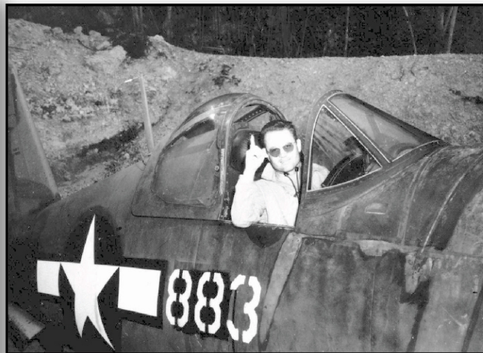
Two photos of Boyington in the cockpit of 883. Note the earlier two-digit side number overpainted (we believe with fresh Dark Sea Blue), and the ragged edges of the numbers "883". It appears a stencil was used, but the paint applied with a brush or roller, resulting in bleed and paint drips. Also note the color of the border on the national insignias.
