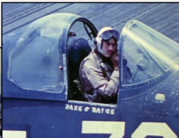
Two stills of "Maze & Hayes". We can only assume the aircraft was named for Maj. Maze and another VMF-511 lost on operations. Note the Gloss Sea Blue paint worn off (?) of the hand hold below the windscreen. No white tip on the prop hub, and the small aircraft numbers were only carried on the upper cowl lip and the forward main gear doors, unlike "My Nel III".
