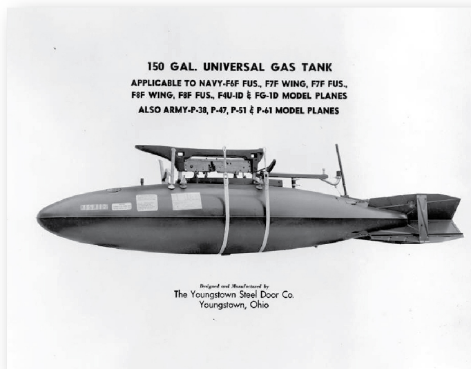
A photo from Youngstown Steel Door Company showing the Mk.5 tank with added fins and straps not fitted to those carried by the F4U.
