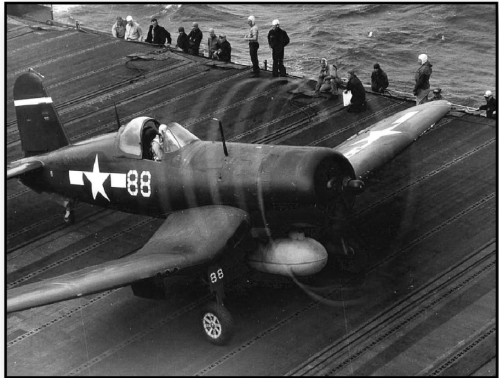
Above: An F4U-1D of CVG-4 launches from the USS Essex in January 1945. The 170-gallon Duramold tank is painted white, a holdover from its previous use on a four-tone camouflaged F4U-1A.
