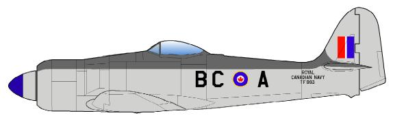
forward). 18" RCN ringed roundels (use the 16" RCN roundel and add a yellow ring) on the fuselage sides and upper wings. Below the starboard wing , **VG** in 36" black letters; under the port wing **BCA**. Royal Canadian Navy and serial number in 4" black solid letters. The spinner had a blue nose cap.
